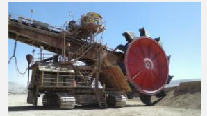
The first teleoperated bucketwheel in the world (2011)
